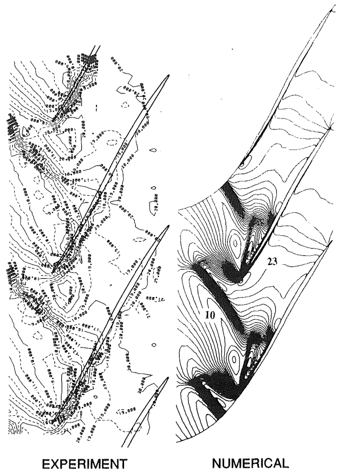
Fig. 4(b) Comparison of casing static pressure at stall condition (90 percent rotor speed)
